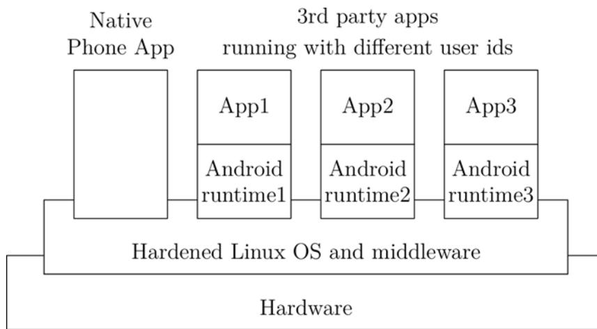
Figure 2 – KaiOS layers. Note that all internal and 3<sup>rd</sup> party apps are web apps and that they are all run by the Gecko runtime
